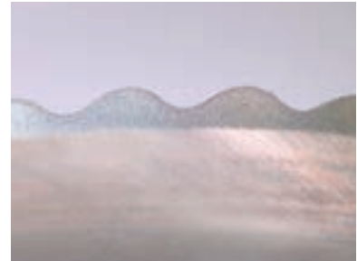
外周刃のラフィング形状 Unequally configured serrations of the cutting edge
