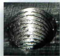
切屑処理→再タップ Once the hole is cleared, tapping can be resumed.
